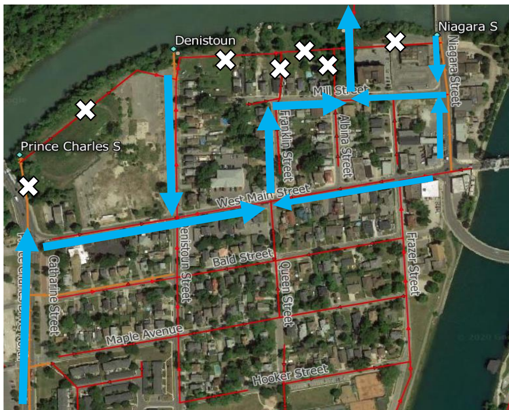
Figure 2 Proposed Network Changes. White X marks represent sewers for abandonment, blue arrows represent new sewers.
