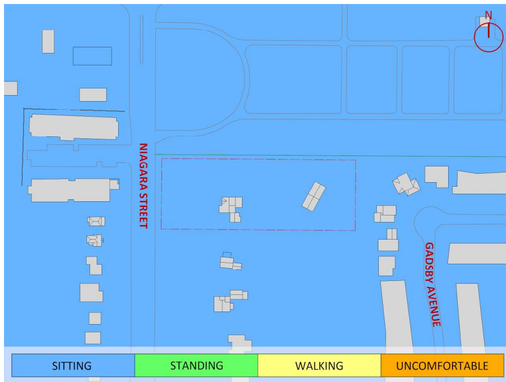
FIGURE 3D: SUMMER – EXISTING MASSING – WIND COMFORT, GRADE LEVEL
