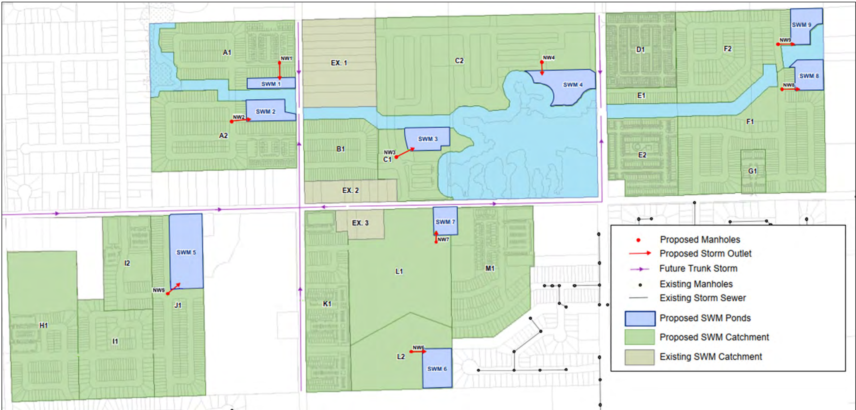
Figure 5-2: Proposed Storm System and Drainage Areas
