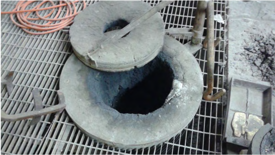
Figure 17 Melting pot for bronze at William Jurgenson Art Foundry Photo N. Reid, Sept. 21, 2017.
