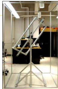
Above: The beam profile is being measured using a custom designed profiler pictured above in its initial construction. The profiler is capable of rotation through three-dimensions to produce a full digital render of a luminaire.
